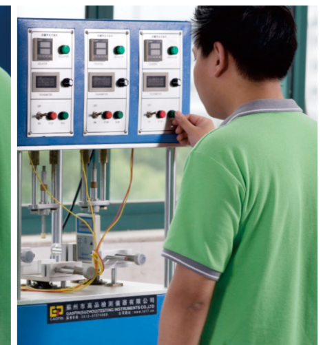
• Key Operation Life Testing Machine
